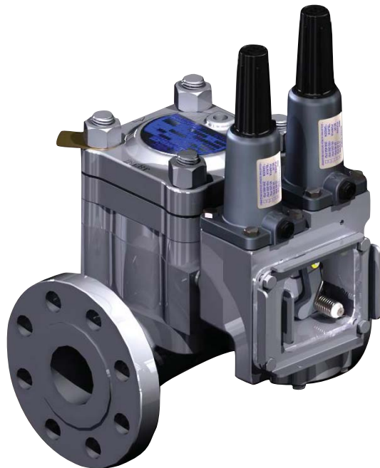
Figure 2 - Two inch Flowgrid Slam Shut regulator with over and under pressure protection.
